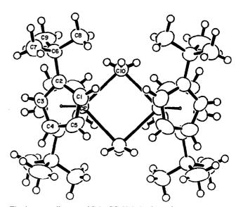
Fig. 1. ORTEP diagram of  $(Me_3CC_5H_4)_4Ce_2(\mu-Me)_2$ . The non-hydrogen atoms represent 50% probability ellipsoids and the refined hydrogen atoms represent arbitrary sized spheres. The hydrogen atoms located on C(1, 3, 4, 5) are numbered H(1, 2, 3, 4), those on C(7, 8, 9) are numbered H(5, 6, 7, 8, 9, 10, 11, 12, 13) and those on C(10) are number H(14, 15).
